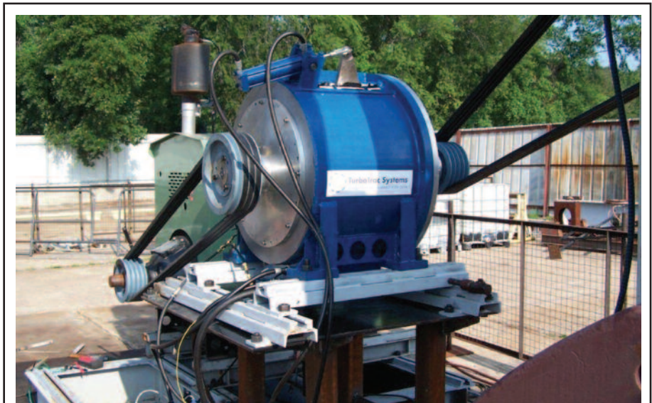
By using Turbo Trac Systems' infinitely variable transmission to connect motors to pumpjacks or compressors, operators can run the motor at a constant speed, but vary the amount of power that reaches the driven device. The company says this eliminates the need for a variable frequency drive while boosting the motor's efficiency and run life.
